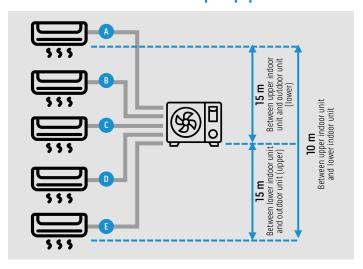
Maximum distance single pipes Indoor unit to Outdoor unit
