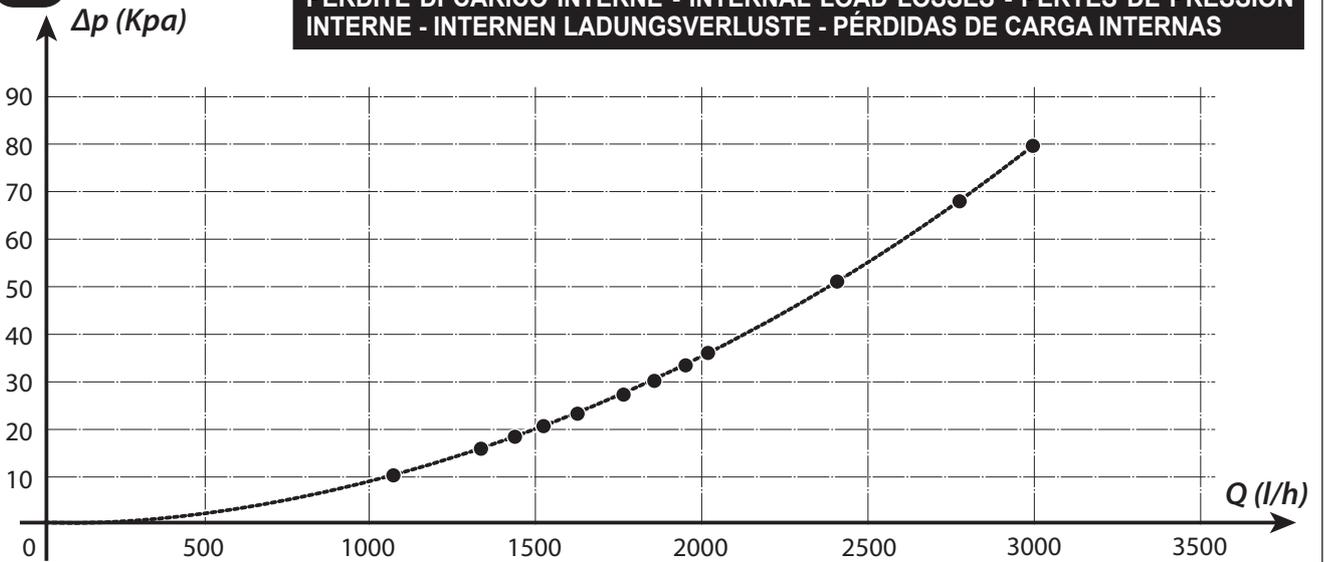
**PERDITE DI CARICO INTERNE CIRCUITO ACS - DHW CIRCUIT INTERNAL LOAD LOSSES - PERTES DE PRESSION INTERNE EN CIRCUIT ECS - WARMWASSERSTROMKREIS INTERNEN LADUNGSVERLUSTE - PÉRDIDAS DE CARGA INTERNAS DEL CIRCUITO ACS**
