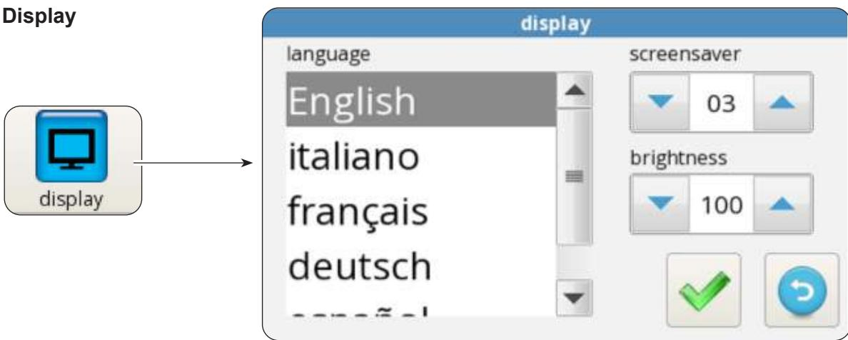
This screen allows to select the language, to set the start delay time of the screensaver function and to set the screen brightness.
